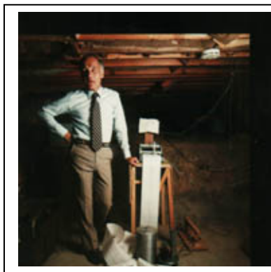
On a level pier in the crawl space of Breiner's basement, the self-made tilt-meter sends its signals to a plotter nearby, registering seismic events as far away as 8,000 miles.
